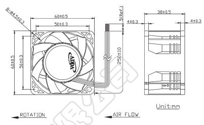
Frame:Plastic(UL:94V-0) Impeller:Plastic(UL:94V-0) Lead wire:UL1061AWG26
