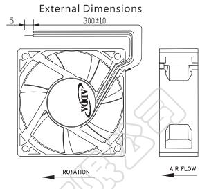
Frame:Plastic(UL:94V-0) Impeller:Plastic(UL:94V-0) Lead wire:UL1007AWG24
